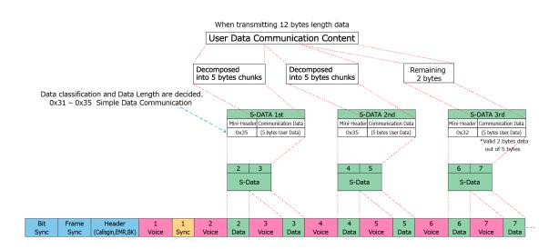
Example: Inserting user data communication content into Radio Format at called side.
