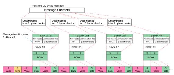
In the above example, the message content is transmitted from "2 Data (data frame 2)" immediately after "1 Sync", but message transmission can also be started from an even number of data frame positions such as "4 Data", "6 Data", or "8 Data".
