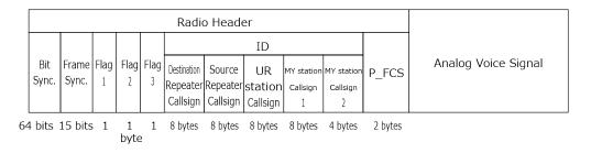
The modulation of the radio header shall be MSK modulation in the voice band, with a transmission rate of 1200 bps, 1200 Hz for signal "1", and 1800 Hz for signal "0".
