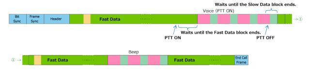
When performing fast data transmission when the PTT is turned off after voice communication has ended (slow to fast), this function is used when high-speed data transmission is desired for a certain period of time after the PTT is turned off, such as in radio applications. (For example, to transmit GPS data when the PTT is off)
