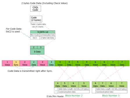
Example of sending the code data of the code squelch periodically during fast data transmission.
