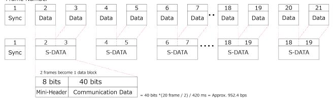
The first 8 bits of the block indicate the data type and data length. This 8-bit is called a miniheader. For this reason, the communication speed by this method is about 950bps.
